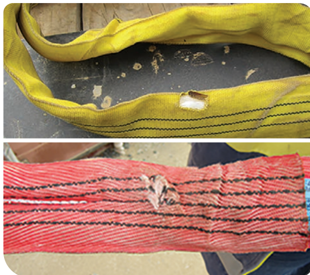
Defective slings to be removed from service
