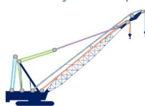
Crawler Crane: Hoist/Auxiliary Hoist Rope
