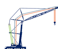
Mobile/Telescopic Crane: Hoist/Auxiliary Hoist Rope
