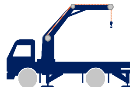
Truck Crane: Hoist Rope
