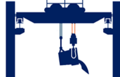
Ladle Crane: Hoist/Auxiliary Hoist Rope
