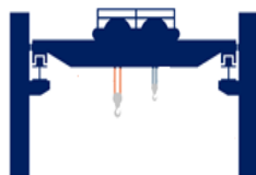
Overhead Crane: Hoist/Auxiliary Hoist Rope
