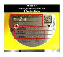
**Step 1.** Locate the model number on the metal identification label (see Photo 1). If your device model number is listed in the table below, proceed to **step 2**. If the model number is not listed below, it is not part of the notice and can be returned to service.
