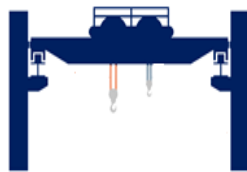
Overhead Crane: Hoist/Auxiliary Hoist Rope
