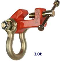
Tiger Bulb Clamp can be side loaded up to 45° and cross loaded up to 15° without derating the unit, whilst still maintaining a 4:1 safety factor.
