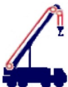
Mobile Crane: Hoist Rope
