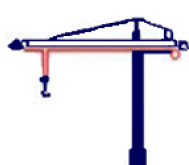
Tower Crane: Hoist Rope
