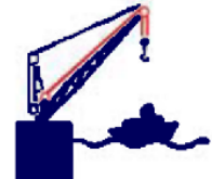
Dock Side Crane: Hoist Rope
